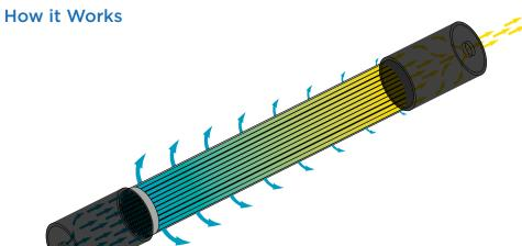
Compressed air, saturated with water vapor, flows through a bundle of tube-shaped hollow membrane fibers. A sweep orifice installed at the end of the bundle meters the amount of sweep air required to remove the water vapor from the dryer. Dry air then exits the tube bundle for use downstream. As long as the dried air isn't exposed to temperatures below the specified pressure dew point, no troublesome liquid water will form in the air system.
